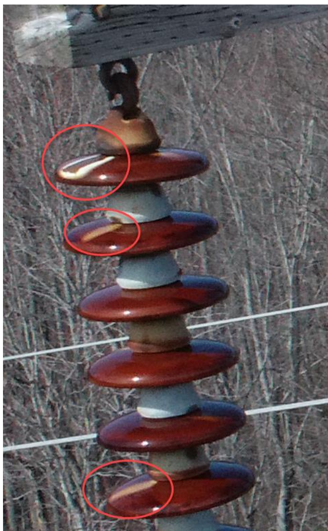
Figure 21: Component 3: Claytor – Fieldale 138-kV Line Structure 30-162: Multiple Flashover/Arcing Damage Indications to Insulator
