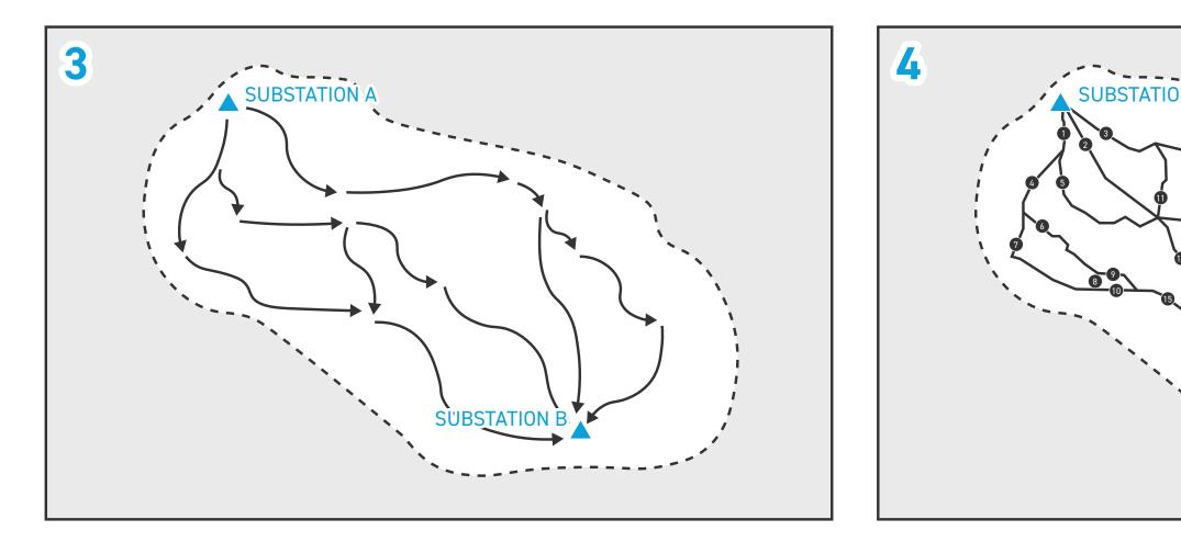
**3. Conceptual Routes:** The routing team uses data gathered to develop conceptual routes adhering to a series of general routing and technical guidelines.
