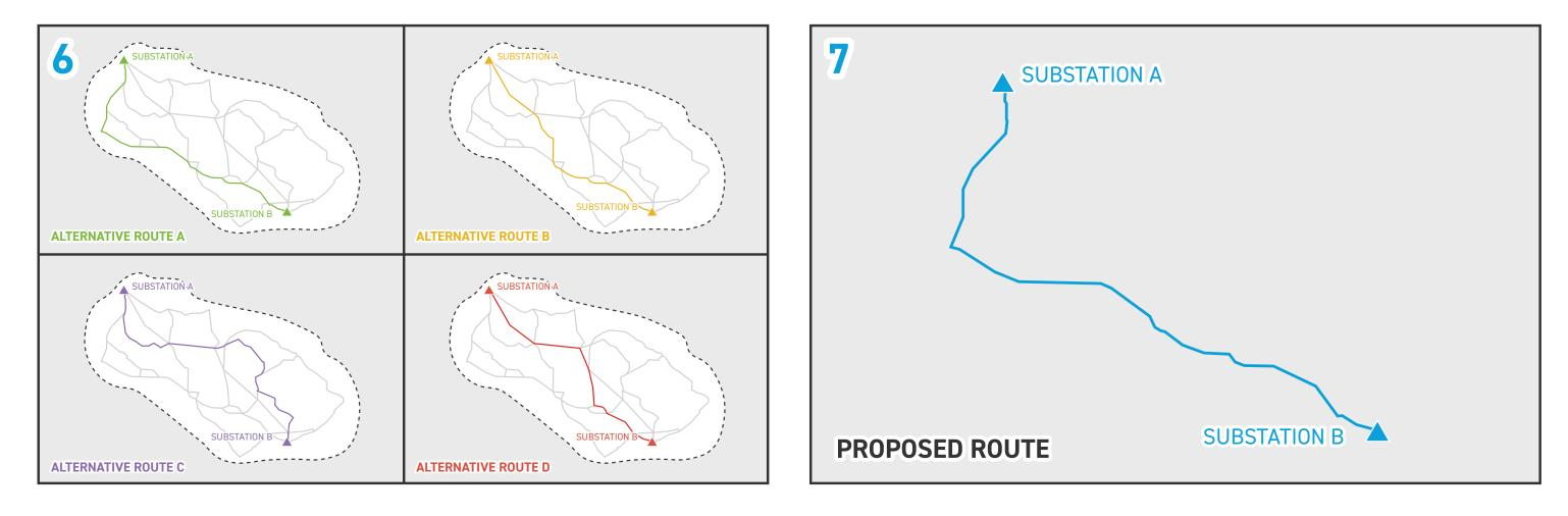
6. Alternative Routes: After public input is gathered, study segments are further refined and evaluated. The most suitable segments are selected and assembled into alternative route options.
