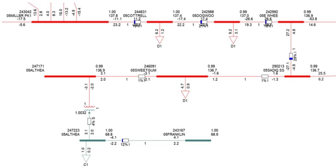
Figure 3-4. System with proposed facility, N-1 loss of Fuller – Argentum (EKPC) 138 kV line
