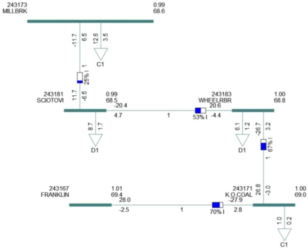
Figure 3-2. System without proposed facility, N-1 loss of Fuller-Argentum (EKPC) 138 kV line.
