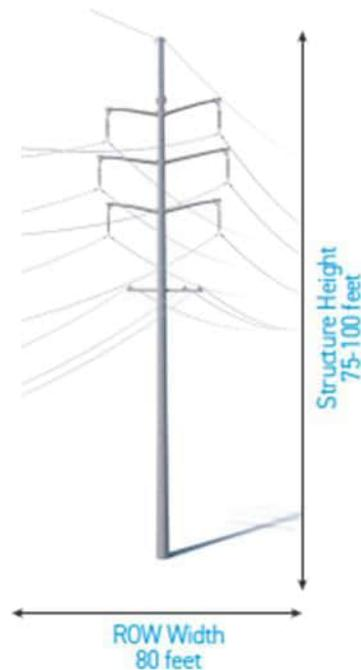
**Figure 2. Typical Transmission Line Structure (Steel Monopole)**
