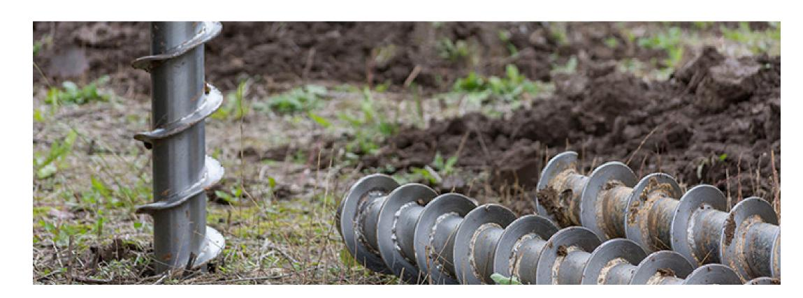
Soil Borings: Field crews use a drill to bring up soil samples and then backfill the holes. Testing the core samples helps determine soil conditions in the area. Soil conditions and types can affect structure location and foundation design.
